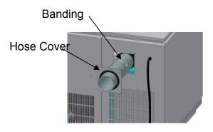
2. Mount the Vent Hose on the Vent mouse and fix the band on it.
