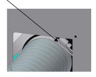
3. Tighten the band by 8mm Spanner or Box Wrench.
